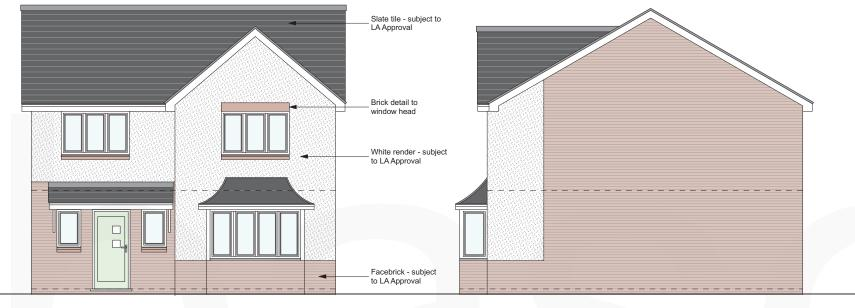
Front Elevation Side Elevation
